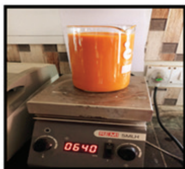
Fig. 2(d). Addition of sodium hydroxide and continuous stirring at 80°C
